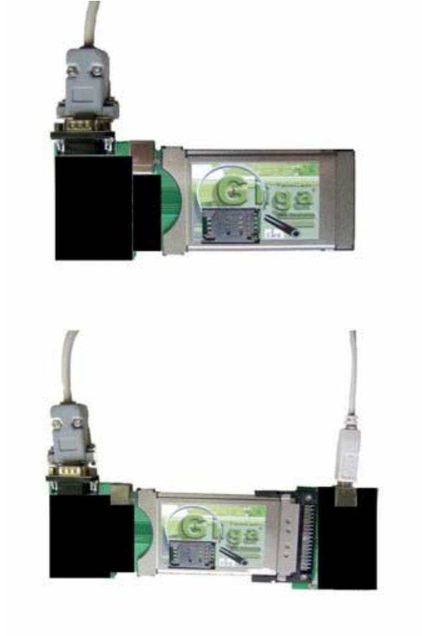
2. Now the Giga PCB must be connected with an USB cable to the PC, this serves for tension care. Connect now the Gigaprogrammer and the PC with a cable RS232 (serial), the cable must be booked 1 to 1, you use no zero modem cable. The USB connection is not required.
