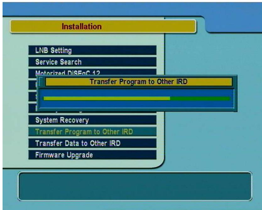
7. Please do not interrupt the download process before complete finish. Even when the process bar reaches the end, the writing process of the flash memory might not be completed and could cause fatal effects. The completion will be shown by displaying 'End' in the display of the front panel. Models without a display indicate the complete procedure by blinking of the green LED on the front panel.
