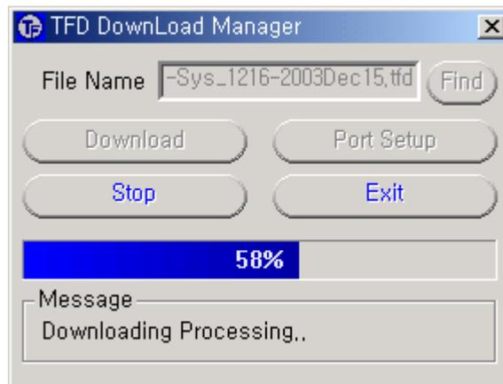
8. Please do not interrupt the download process before complete finish. Even when the process bar reaches the end, the writing process of the flash memory might not be completed and could cause fatal effects. The completion will be shown by displaying 'End' in the display of the front panel. Models without a display indicate the complete procedure by blinking of the green LED on the front panel.
