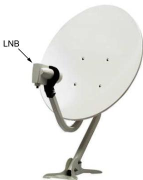
The LNB (Low Noise Block converter) is used to take a wide band of relatively high frequencies, amplify and convert them to similar signals that is carried at a much lower frequency, which is called Intermediate Frequency (IF). High frequencies from satellites are converted into 950 to 2150 MHz by a LNB.
